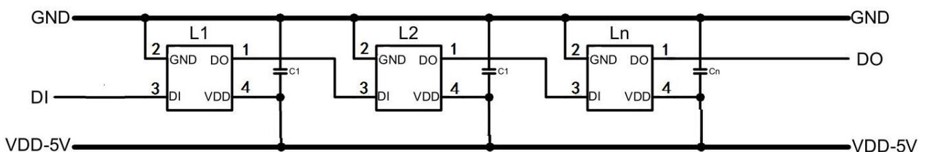
Remarks: C1 is the filter capacitor for VDD, its value of 100NF.
