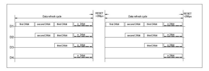
Note: The data of D1 is sent by MCU, and D2, D3, D4 through pixel internal reshaping amplification to transmit.
