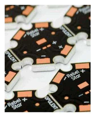
This is a custom MCPCB structure that further enhances heat dissipation and thus enabling the LED to last according to its life time.
